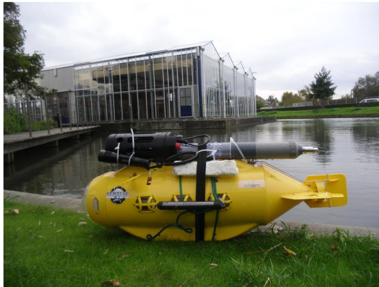
Figure 4 Underwater drone equipped with water quality sensors (multi-parameter probe on top and CTD on the side) and with HD video cameras (at the front).
